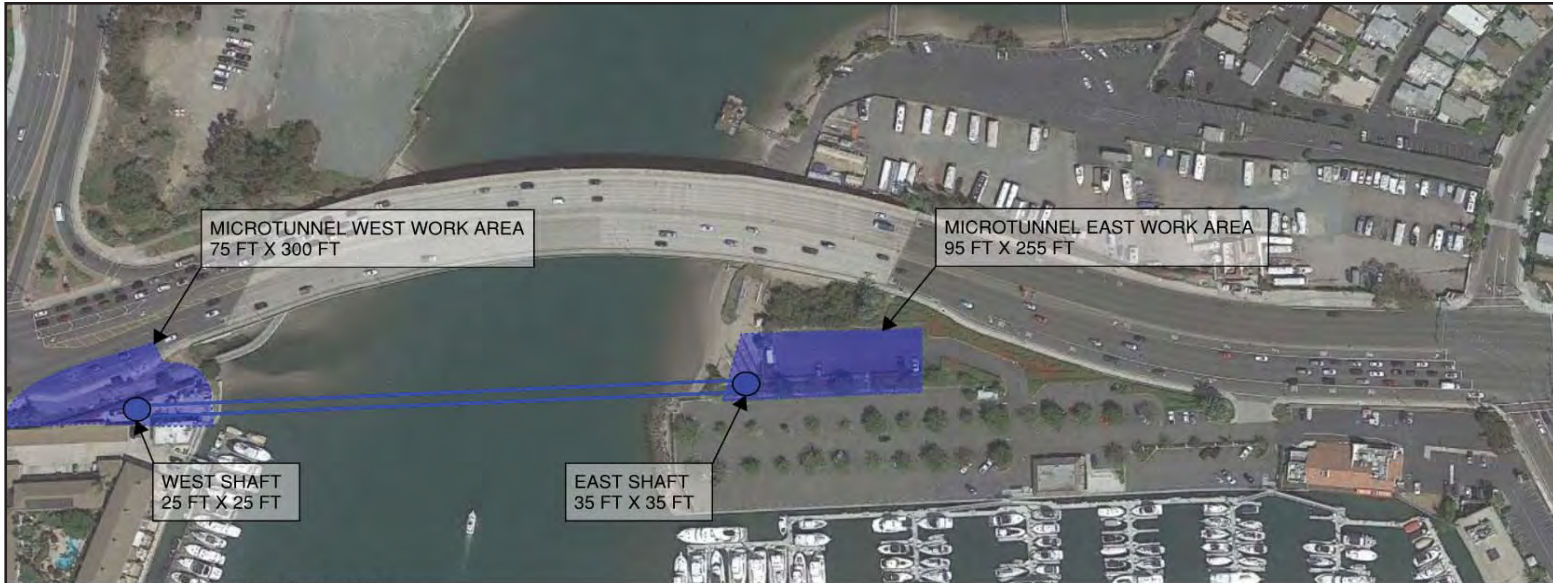
Newport Bay Channel Crossing Work Areas
